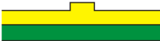
1.4 \mu\text{m} rib waveguide R \sim 1 \text{ mm} \alpha \sim 0.2 \text{ dB/cm}
